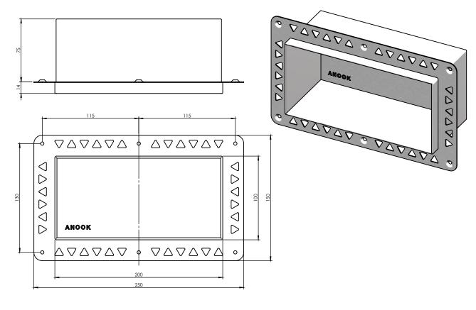
**NOTE:** Each side has 1 degree of fall to stop water pooling.
