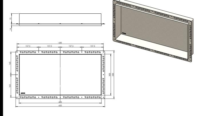
NOTE: Each side has 1 degree of fall to stop water pooling.
